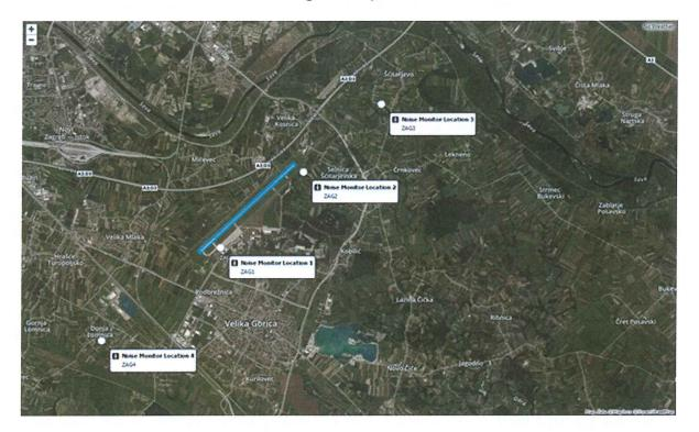
Two fixed measuring devices are close to the edges of runway 04 and 22. Distance of station NMT 1 from edge of runway 04 about 306 meters, distance of station NMT 2 from edge of runway 22 about 307 meters.
