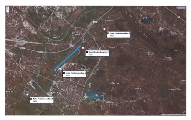
Two fixed measuring devices are close to the edges of runway 05 and 23. Distance of station NMT 1 from edge of runway 05 about 306 meters, distance of station NMT 2 from edge of runway 23 about 307 meters. The third and fourth station are fixed devices set at settlement Obrezina and Donja Lomnica. The portable device has its own power supply, which can be transferred to any location around the airport.
